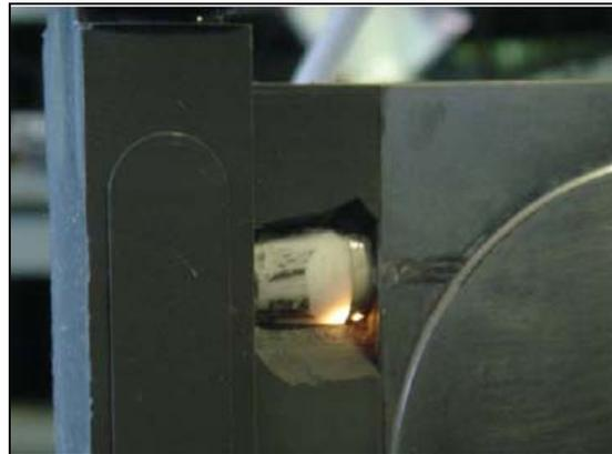
**Figure 5: Cooling device with sidewall leakage**
