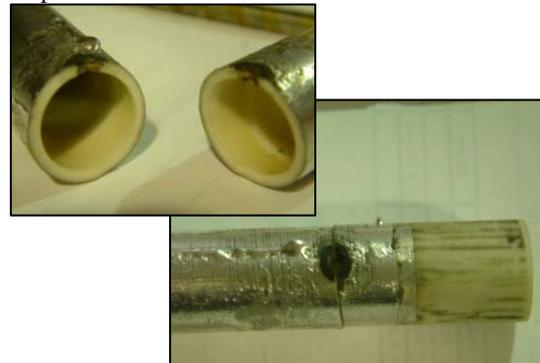
**Figure 4: Cooling Device failed Ceramic tube**
