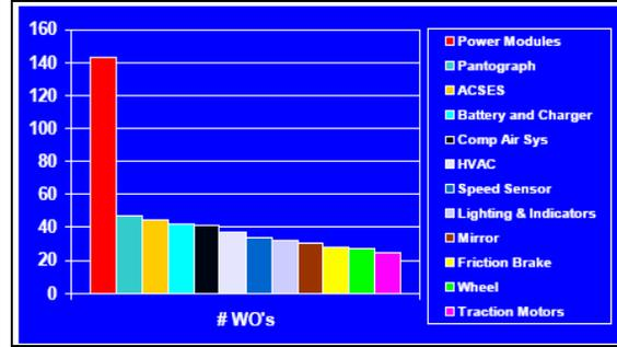
Figure 2: Failure data for HHP-8 fleet
