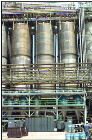
Figure 11.1: Product Silo with Blend Tubes
